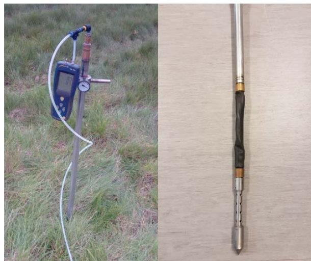
Fig. 4. Active probe in the borehole, on the right the pressure balloon for sealing is seen.
