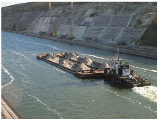
Fig. 3. The pushed formations carrying coal and aggregates on the Gliwicki Canal and the Rhine respectively [5, 8]
