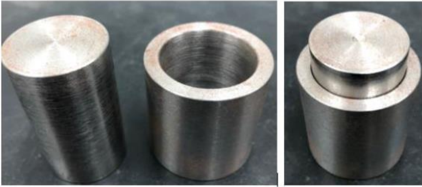
Fig. 5. Piston–cylinder system for the Poisson's effect reduction
