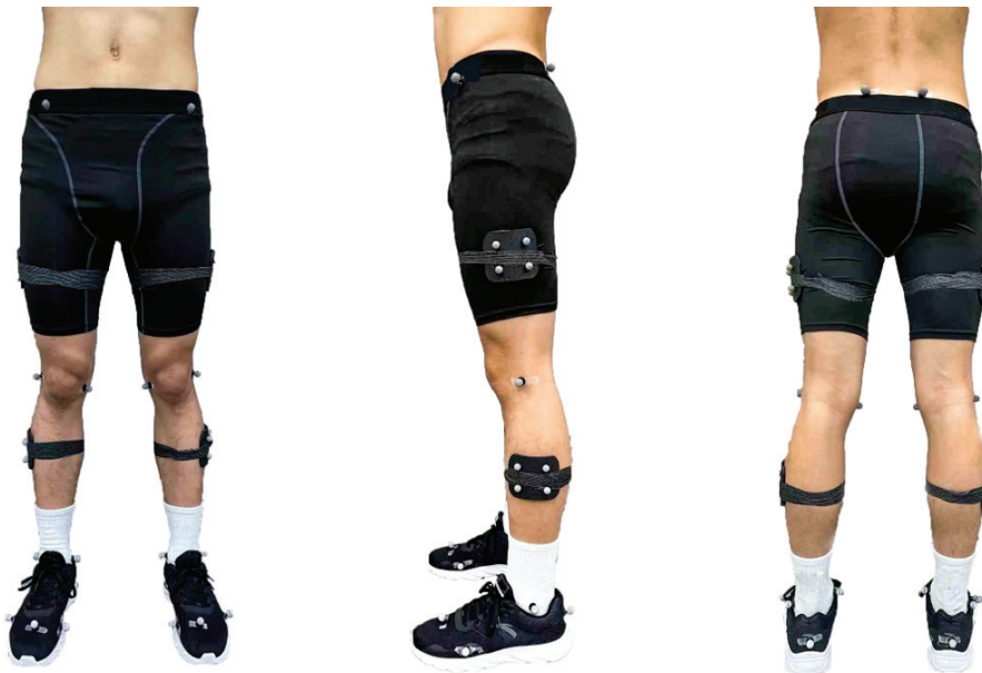
Fig. 1. Illustration of retroreflective marker placement
