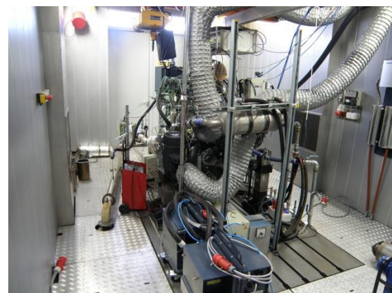
Fig. 2. Engine with exhaust line set up in Engine Testing Laboratory, BOSMAL Institute
