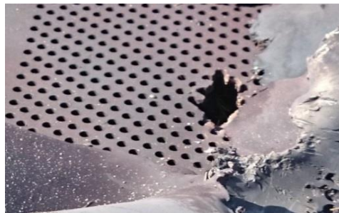
Fig. 3. Example photographs of the armoured panel perforated steel sheet fragments at (A) the explosion area of the PG-7 RPG and (B) superplastic jet entry
