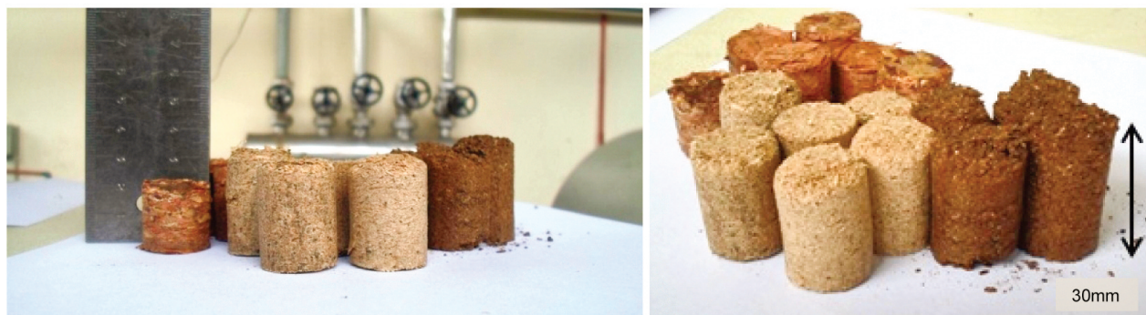
Figure 3. Pellets from sawdust, coconut shells and wood shavings made by pressing.
