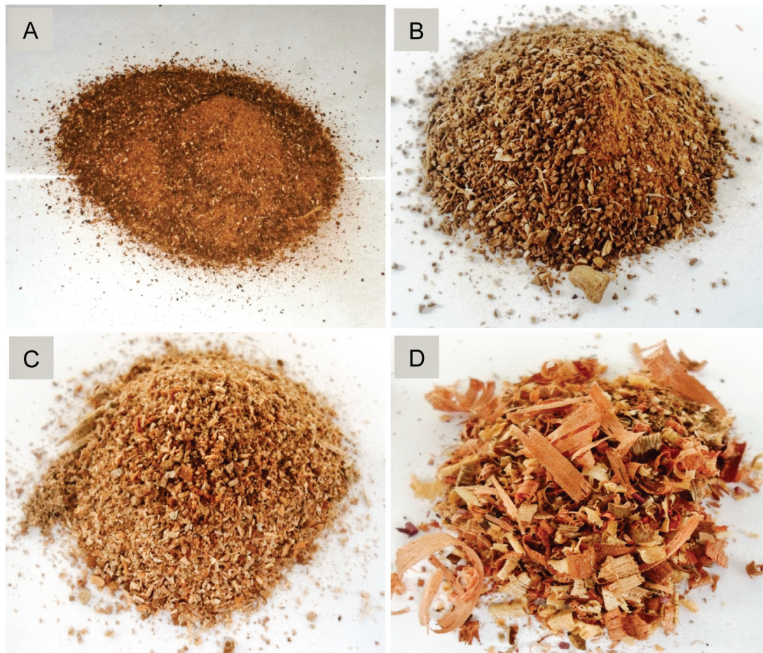
Figure 2. Biomass employed for solid biofuel production after pretreatment: A-oil palm shells, B-coconut shells, C-sawdust, D-wood shavings.
