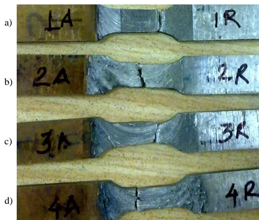
Fig. 4. Fracture location of the four samples
