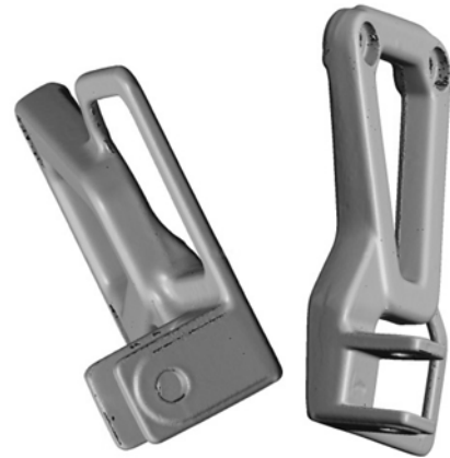
Fig. 5. Unscanned places of the part (black color)
