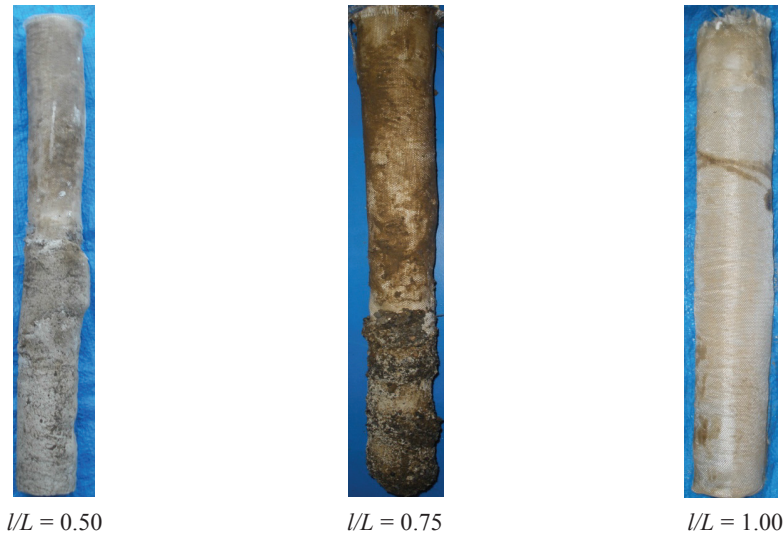
Fig. 20. Deformed shapes of ESCs for different l/L ratios.
