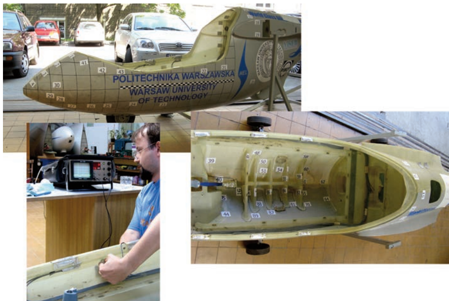
Figure 10. Examination of the fuselage structure after the Test 1
