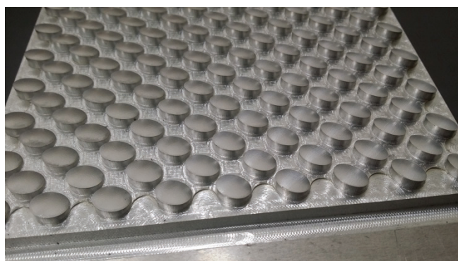
Fig. 4. Model of target to measuring the angle of reflection of infrared radiation
