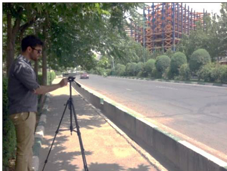
Fig. 1. Placement of sound level meter near the edge of carriageway
