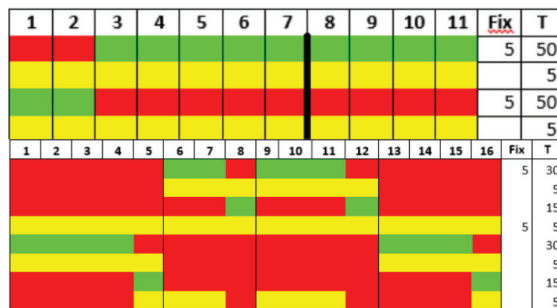
Fig. 5. Sequence tables for (a) two first simple intersections (Bajana str. and Hutnicza str.), (b) a more complicated intersection (Na Ostatnim Groszu str.)
