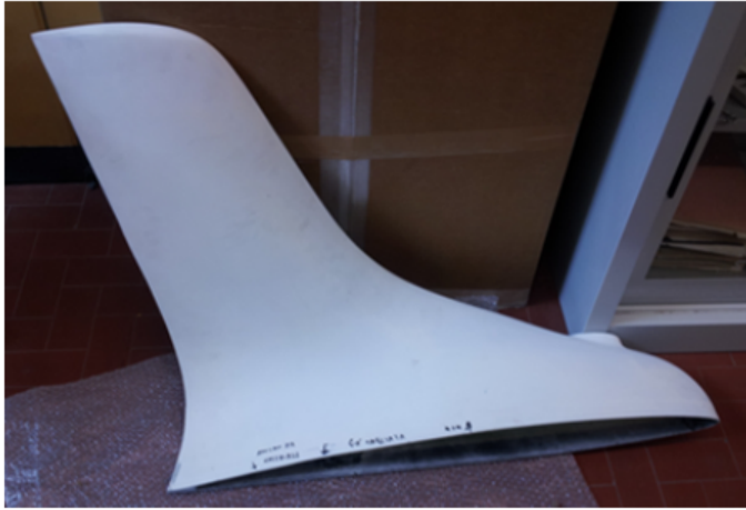
Fig. 1. The investigated composite full scale blended winglet
