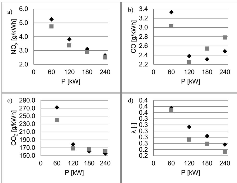
Fig. 4. The results of the a) NO<sub>x</sub>, b) CO, c) CO<sub>2</sub> emissions and d)  $\lambda$  for all considered loads and observations: ◆ – the engine assumed as operated without malfunctions, ■ – throttling of the intake air duct
