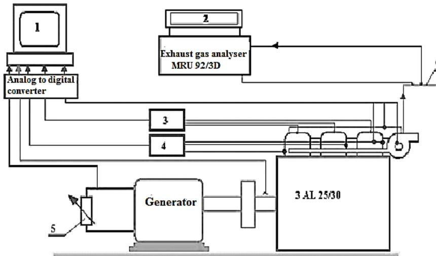
*Fig. 1. The laboratory stand diagram elaborates [4]: 1 – computer – recorder, 2 – exhaust gas analyser 3– combustion pressure indicator, 4 – injection pressure indicator, 5 – water resistance, 6 – exhaust duct*
