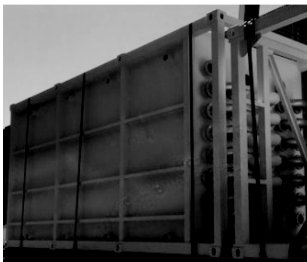
Fig. 2. Pyrolysis plant PTR 1000 kW6 (HEDVIGA GROUP plc) – cooling module [3]
