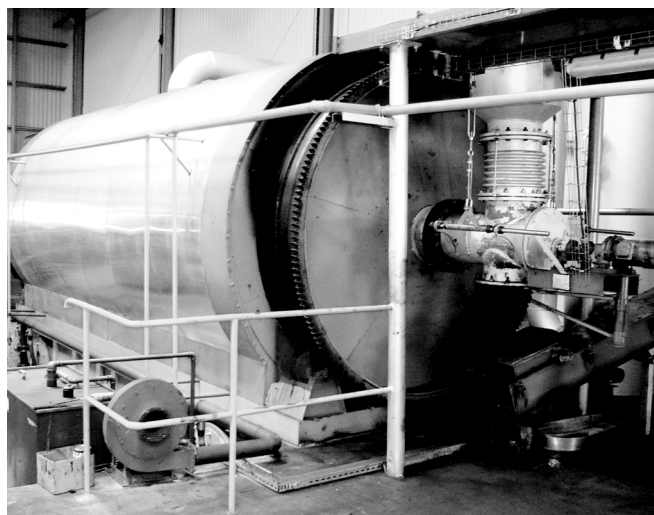
Fig. 1. Discontinuous pyrolysis plant (batch process) of company Shangqiu Jinpeng Industrial Co., Ltd. – reactor or rather rotary pyrolysis kiln (photo - author)
