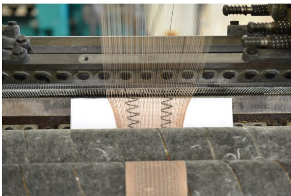
Fig. 14. Technology of manufacturing a knitted strip with carbon threads on a warp-knitting machine Karl Mayer type RL5NF
