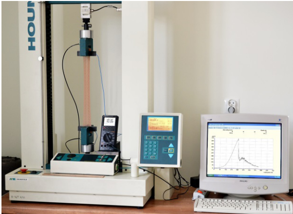
Fig. 17. Methodology of measuring resistance changes of electrically conductive threads in the process of stretching a knitted strip
