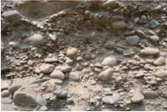
Fig.2 Sandy Cobble Stratum with High Content of Big-sized Cobble
