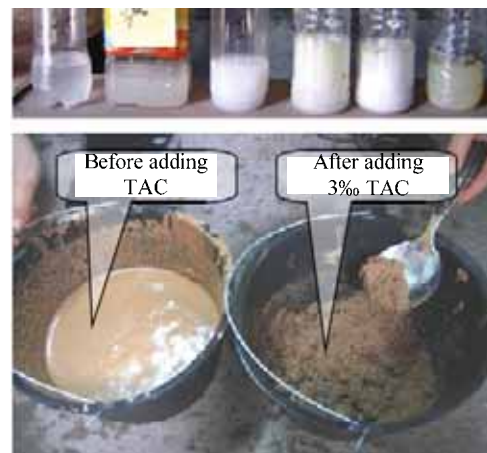
Fig.3 The appearance and experimental results of TAC polymer
