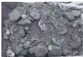
(a) Sandy cobble soil after digging and mixing
