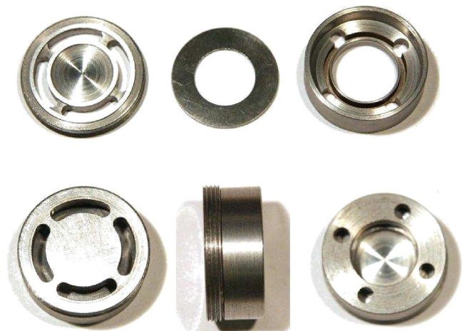
Fig. 21. Prototype of the ring valve worked out for the oscillatory compressor
