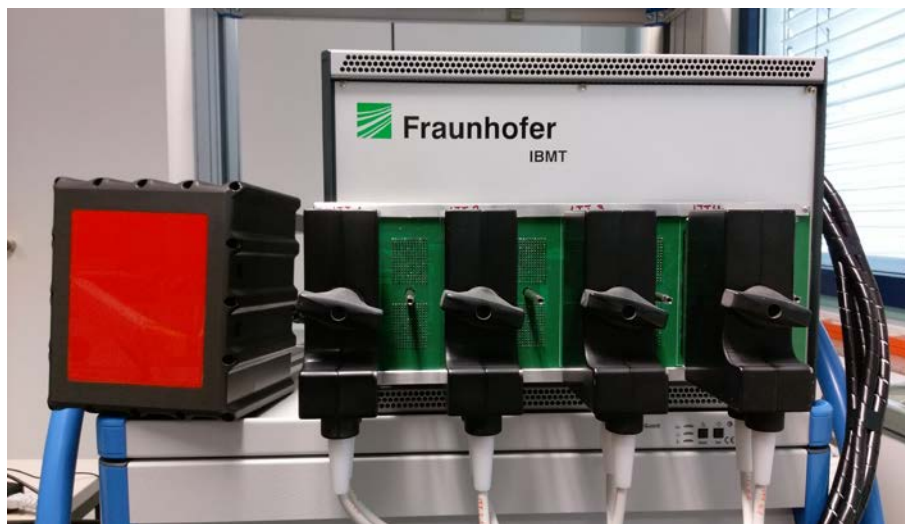
Fig. 14. Experimental setup of the 3D sonar camera system
