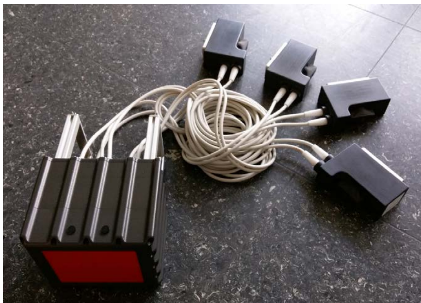
Fig. 8. 3D sonar camera with connecting cables of 2 m length.
