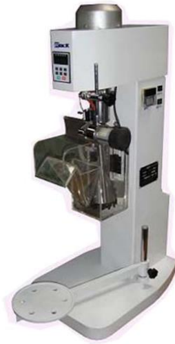
Fig. 2. Actual diagram of experimental system for mechanical flotation tests
