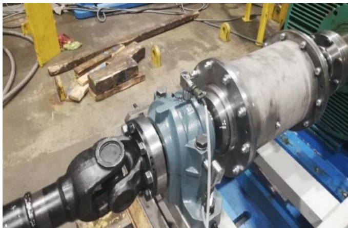
Fig. 6. Flexible clutch mounted on the test rig (source: authors' contribution).
