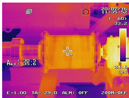
Fig. 29. Thermograms of the flexible clutch subject to tests, as determined in the durability tests.
