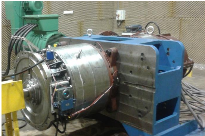
Fig. 2. Planetary gear transmission with an ATEX-compliant technical diagnostic system installed inside the housing while in testing (source: authors' contribution).
