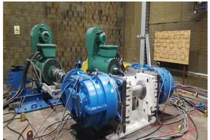
Fig.8. Gear transmissions mounted in a scraper conveyor body (source: authors' contribution).
