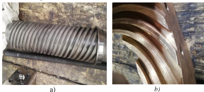
Fig. 28. Surface of the bolt (a) and of the nut (b) following the durability tests.
