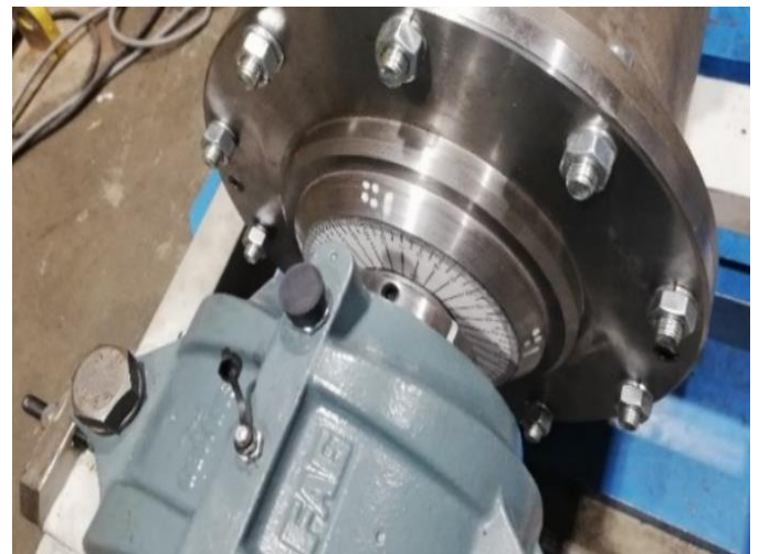
Fig. 9. Measuring disc while determining the static characteristics of the highly flexible clutch (source: authors' contribution).
