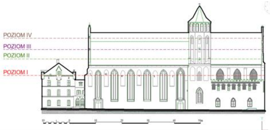
Fig. 8. Vertical (longitudinal) section through the Basilica of St. St. Mikołaja in Gdańsk with marked levels of measuring sensors placement ( own elaboration ) [50]
