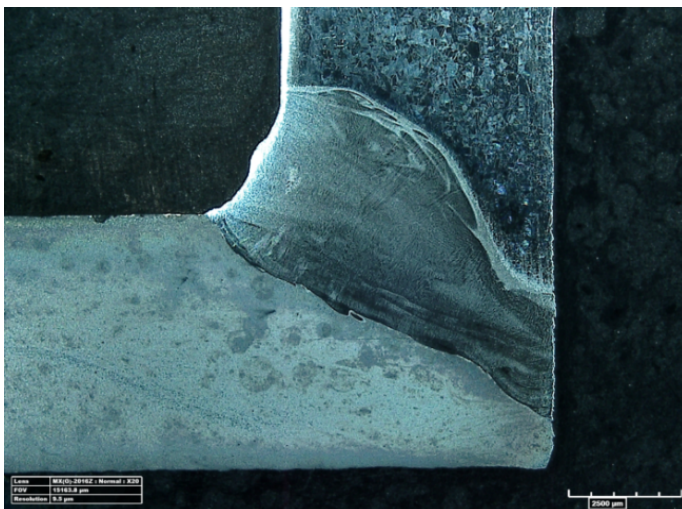
Fig. 7. Fusion zone in cross section – experimental and simulation result
