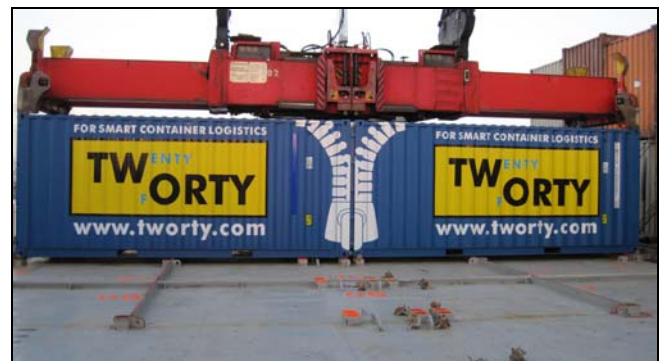
Figure 1. A pair of Tworty Boxes is loaded in Hamburg in coupled condition on board the "OOCL Montreal"
