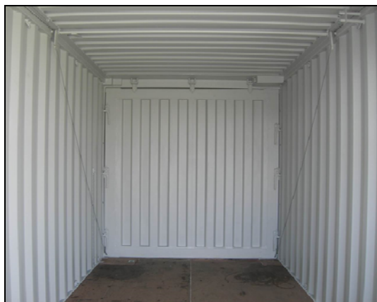
Figure 3. Inside view of closed additional front side door (cables to open the door are visible).
