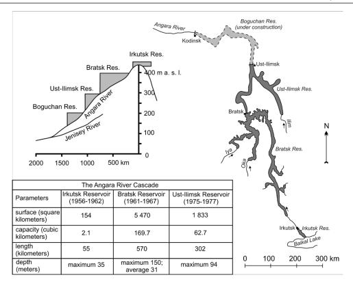
Fig. 1. The Angara reservoir cascade scheme, the main parameters Source: Ovchinnikov et al. 1999
