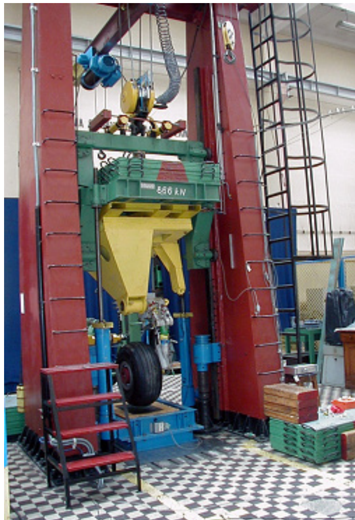
Fig. 5. Landing gear drop test machine example – measurement plate is below the landing gear, source ILOT
