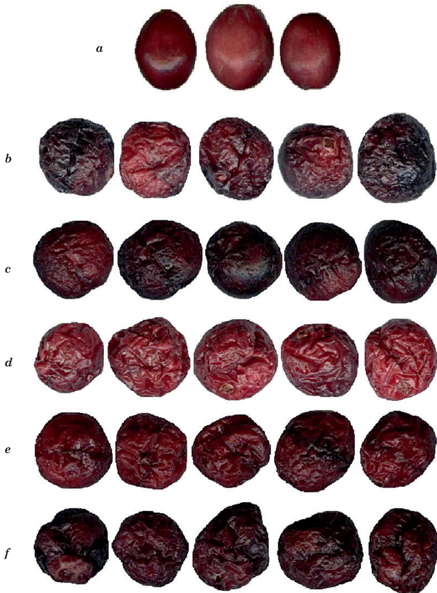
Fig. 3. The overall appearance of: a – raw cranberries (R), b – raw (non-treated) fruits subjected to osmo-microwave-vacuum drying (ROM), c – fruits subjected to sonication and osmo-microwave-vacuum drying (SOM), d – fruits subjected to convective freezing and osmo-microwave-vacuum drying (FOM), e – fruits subjected to sonication combined with convective freezing and osmo-microwave-vacuum drying (SFOM), f – fruits subjected to cryogenic freezing and osmo-microwave-vacuum drying (NOM)
