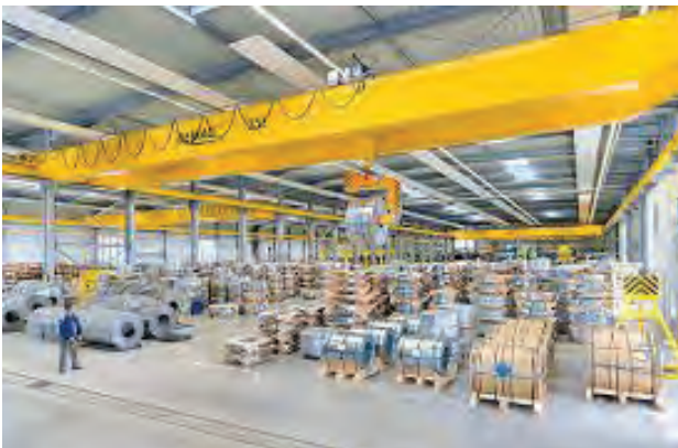
Fig. 2. Industrial steel building with a handling system [2]
