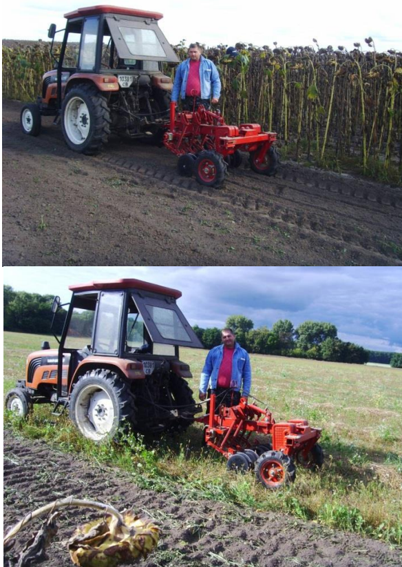
Fig. 9. Functioning of the device for determining the conductive properties of the soil environment on different types of agricultural background
