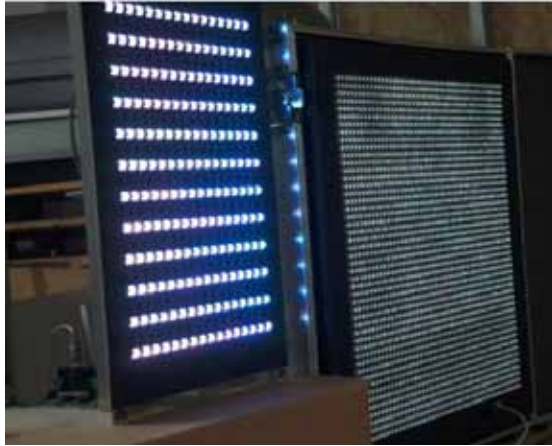
Fig.11. The effects of changes in the colour, depending on the angle of observation – on the left is the classic RGB, on the right the 3G optics.
