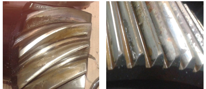
Fig. 4 Examples of gear wheels damaged by pitting
