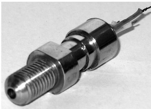
Fig. 5. External inspection of the pressure sensor
