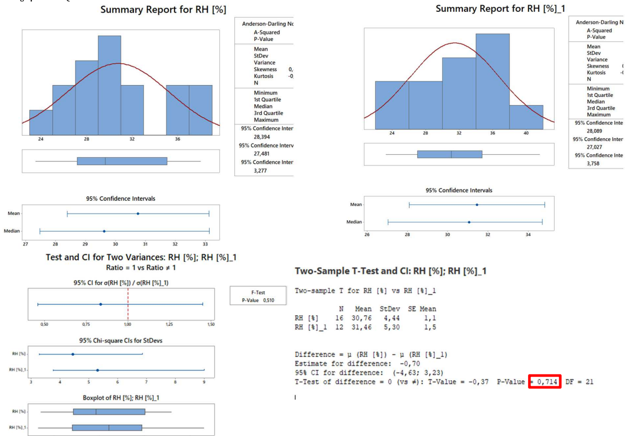
Fig. 14-16 Testing of the normality of product group distributions along with the F – test on homogeneity of variance and comparison of the mean values of relative humidity \bar{x} distributions using the t–Student’s test for Good v. Bad groups of products. Source: own research.
