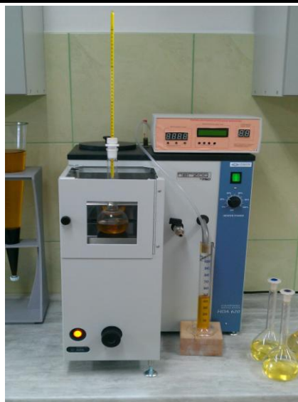
Fig. 2. Photo bench equipped with a distiller HAD 620/1 by Herzog
