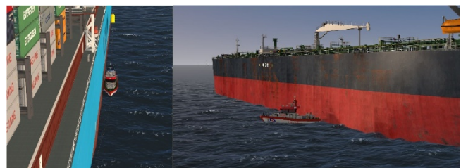
Figure 4. Visualization of service watercraft equipped with Mobile Electromagnetic Mooring System during mooring operations. Source: Authors' own study carried out on manoeuvring simulators of the Gdynia Maritime University in December 2022.
