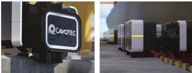
Figure 2. Automated Mooring System – Moor Master - Cavotec. SOURCE: MoorMaster:[ https://www.moormaster.com ], [28]. Accessed on 20.03.2023
