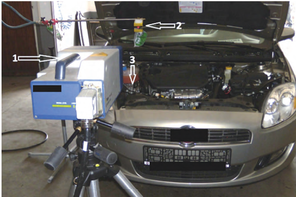
Fig. 3. LDV acquisition in progress: 1- laser probe, 2- mirror, 3- place of laser beam reflection
