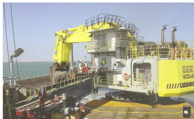
Fig. 5. Backhoe dredger (excavator) [14]
