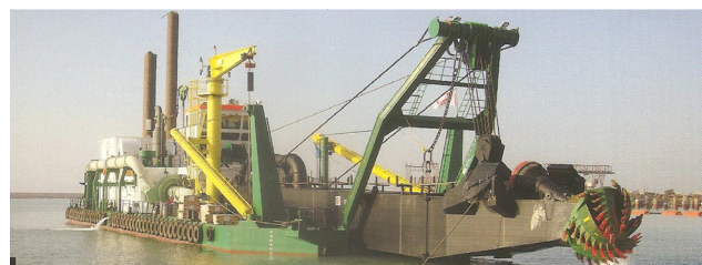
Fig. 2. Cutter suction dredger, trailing [13]
