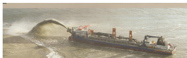
Fig. 6. TSDH dredger forming new land[13]
