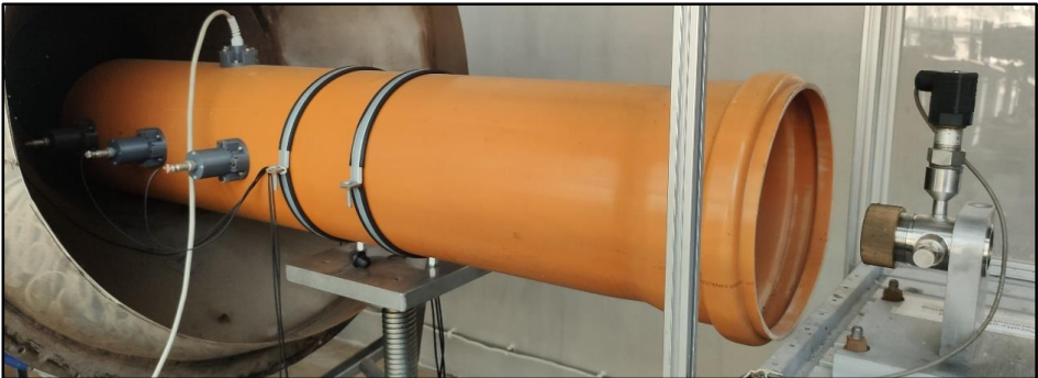
Fig. 2. Test stand: the test chamber with a laboratory rocket micromotor
