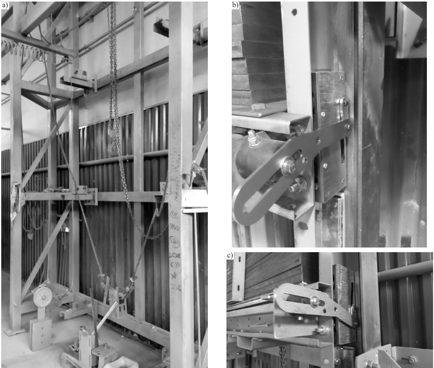
Fig. 8. The test stand: a) general view of the stand for experimental test, b) the progressive gear with the loading system in the neutral position, c) the progressive gear with the loading system at a given load
