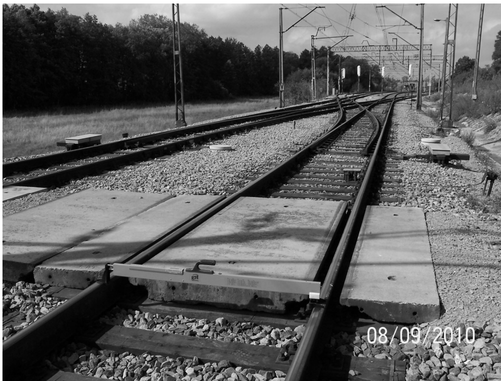
Fig. 2. Surveying the geometry of turnouts and crossover in Słomniki station with a self-recording track measurement gauge RTE2 PROVENTUS.
