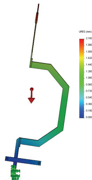
Fig. 16. Results obtained from the simulation of the displacements of the individual points on elements of the measuring instrument mounted at the end of the measuring instrument on the side opposite to the measuring assembly, vertically with measuring assembly up, variant B of the bow cross-section [the author's own elaboration]
