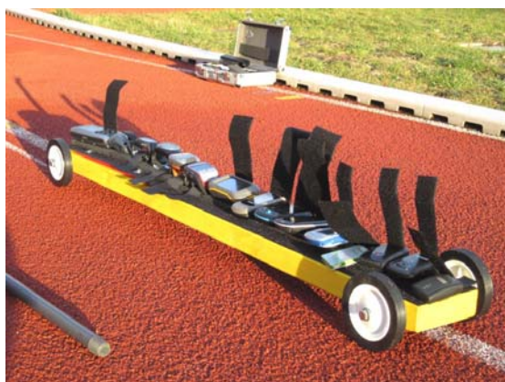
Fig. 10. Arrangement of devices on the measuring trolley [own study]
