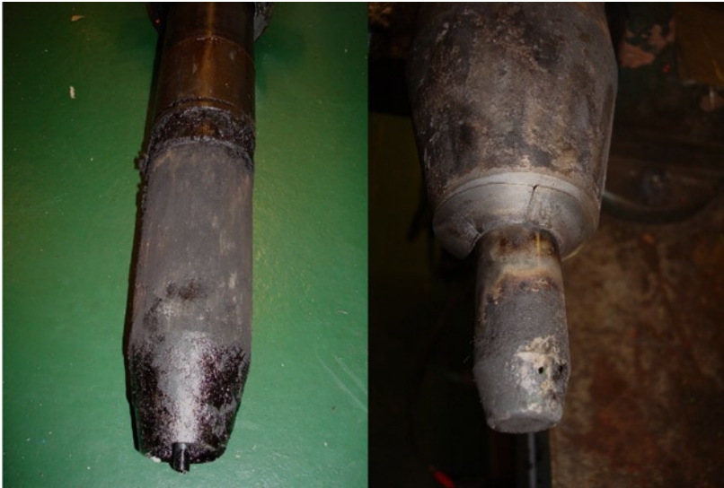
Fig. 2. FIV nozzle tip damages assigned to the high risk failure group: left-hand photo – failure not related to SECA fuel changeover; right-hand photo – failure related to SECA fuel changeover
