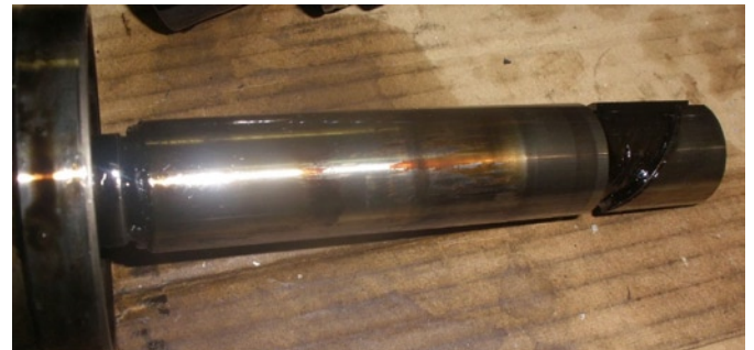
Fig. 5. Fuel injection pump plunger seizure occurred during rapid fuel changeover from residual to low sulfur distillate fuel
