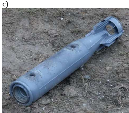
Fig. 9 Configuration testing: two EGP type II devices - bomb No. 4 (shot 6): a - detailed view of the positioning of the EGP device situated at the distance 10 mm from bomb surface, opposite its TNT charge, b - position of two EGP type II devices in relation to bomb surface, c - effect of two EGPs on bomb.
