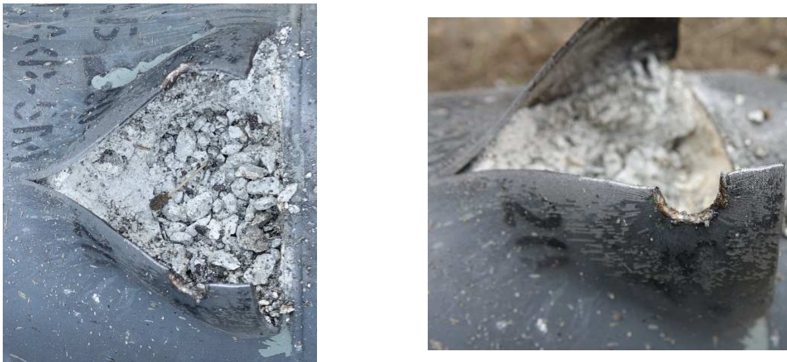
Fig. 7 Detail view of the perforation and local bursting of the front part of the bomb No. 2 body and the penetration and shattering of the TNT charge by the EGP type I device (shot 4): a - top view, b – in the foreground, a view of the edge of the sheet metal of the bomb body with an arched fragment, indicating that the perforation of the body in the form of a circular hole took place first, followed by its bursting.
