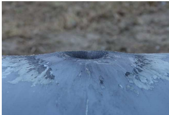
Fig. 10 Detailed view of the perforation of the rear part of the body of bomb No. 4 by the EGP from EGP device type II (shot no. 6): a - top view, b - side view.
