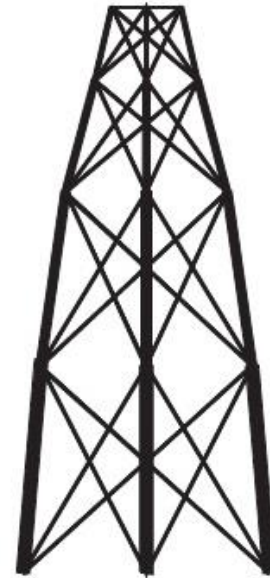
Fig. 2. Optimal shape 39-bar truss
