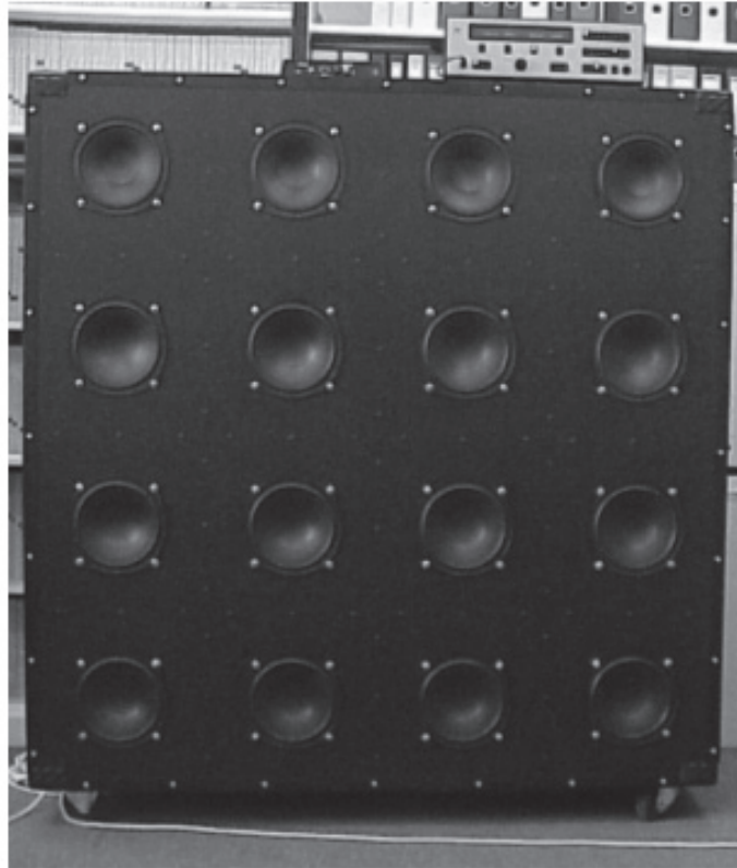
Figure 7. An acoustic model of a power transformer.
