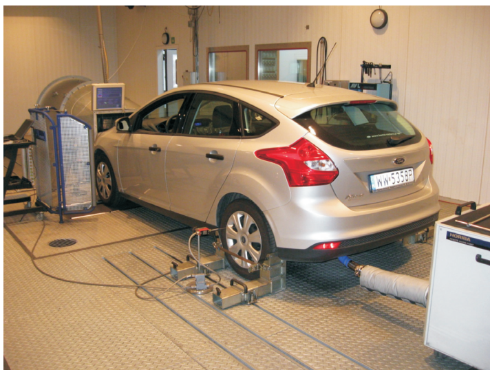
Fig. 2. Exhaust emissions laboratory at BOSMAL Automotive R&D Institute, showing the chassis dynamometer, windspeed fan and a vehicle, all within the climatic chamber
