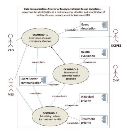
Figure 5. Diagram of use cases of DCSMMRO components for the identification of a post-emergency situation and prioritization of victims of a mass casualty event for treatment in HED (source: own elaboration)
